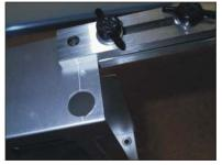
Step 2.1 : Mark the  $T_c$  dimension on each side of the avionics tray. A precise way to do this is to set a dial caliper to the  $T_c$  dimension, lock it in place, and use the tray's edge as a guide to lightly scribe a line on the tray surface.
