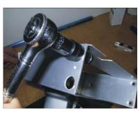
Step 2.2 : Slide the RT500 into place on the tray and line up the index mark on the side of the tool with the  $T_c$  centerline. Verifying that the lower portion of the tool is seated firmly against the edge of the tray with the "foot" slid over the tray's edge, lock the tool in place with the included allen wrench. Drill the pilot hole with the included drill bit.
