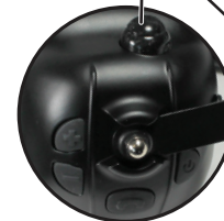
The PTT button on the BTH-900 is different than the BTH-700 and BTH-800.
