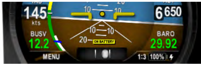
Figure 67: On Battery Operation
