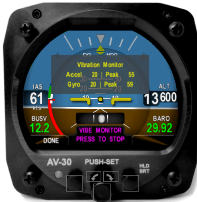
Figure 110: Vibe Monitor Operation
