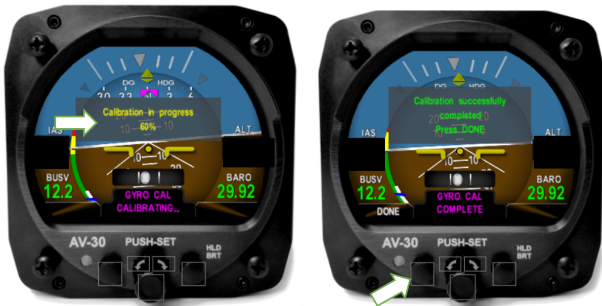
Figure 97: Gyro Calibration Procedure
