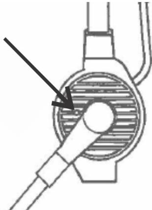
**FIGURE 2.** Gain Adjustment Control
